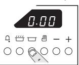
required 'Stop Time' shows. AUTO will show in the display. When your cooking is finished the beeper sounds. TURN THE OVEN KNOB TO 0 FIRST, then press once to stop the beep, press again to return to manual cooking.
